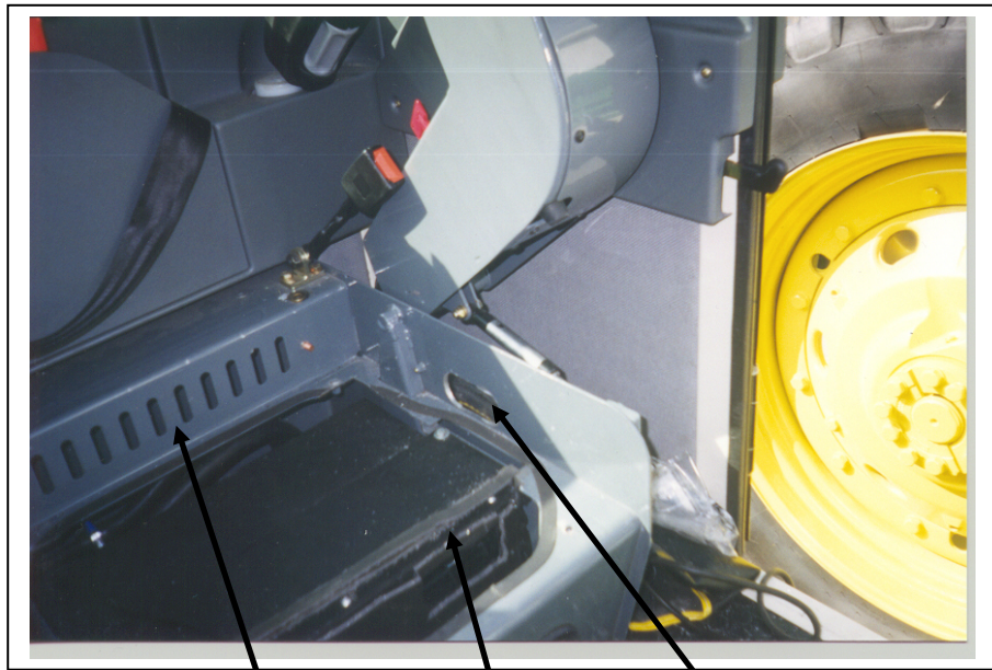
Inside air panel removed
