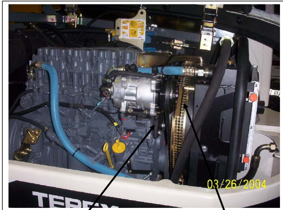
Main mount plate installed. Bolt it to the engine and the angled stiffener bracket. Use the supplied M10 bolts to attach it to the engine and the 3/8" x 1" bolt for the angled stiffener.
