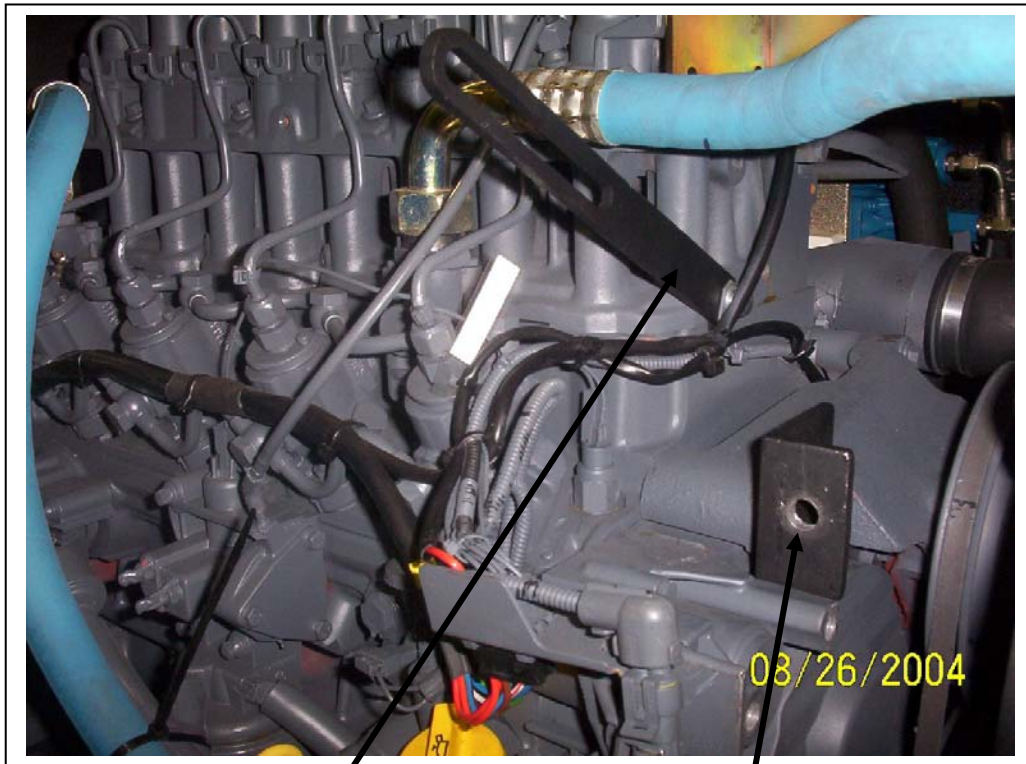
Angled stiffener bracket in place using the longer M8 bolt supplied.
